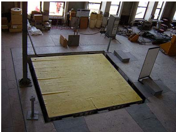
Figure 1. The biaxial shaking table
