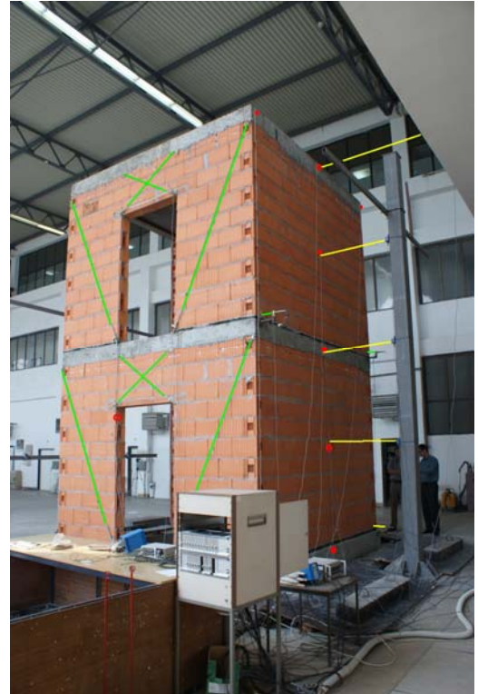
Figure 4. Typical test model of building
