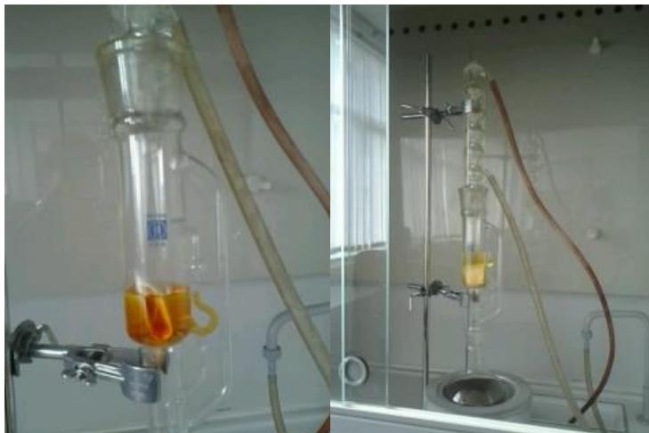
*Figure 2. Soxlet apparatus for extraction*
