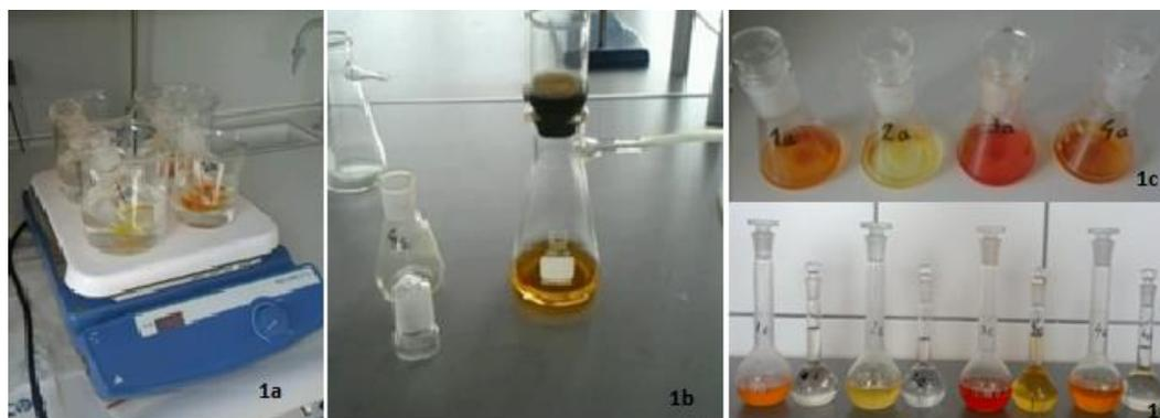
**Figure 1. Phases of vacuum filtration method for extracting the oleoresins (1a maceration; 1b vacuum filtration; 1c and 1d dilution of oleoresins)**
