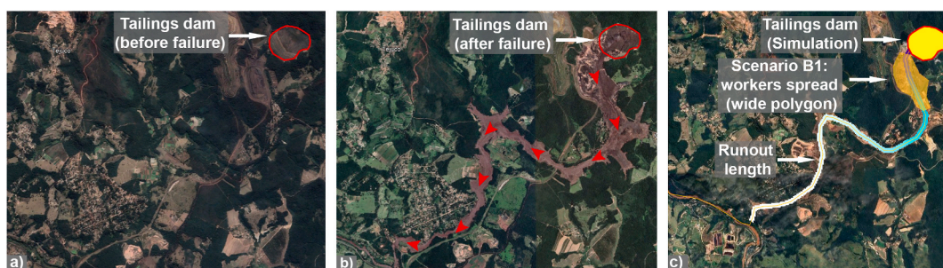
Fig. 9. Brumadinho (2019) tailings dam failure: (a) pre-failure setting, (b) post-failure inundation footprint, and (c) modelled hazard corridor (Scenario B1).
