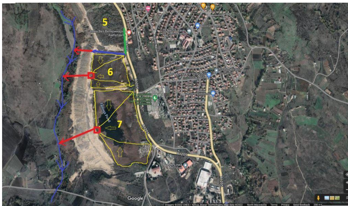
Figure 4. Layout of Probištip Tailings Ponds 6 and 7 and the Side Tailings Embankment Parallel to the Kiselická River [6]
