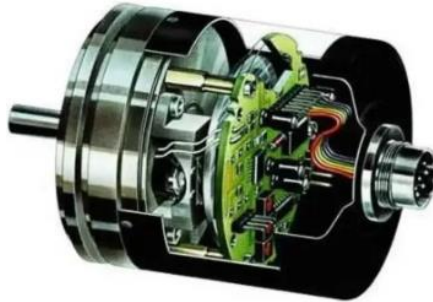
Fig. 1 An optical rotary encoder [1]
