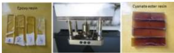
Figure1: Samples prepared from both of thermoset matrices and the sample holder used in the DMA instrument for 3pbt
