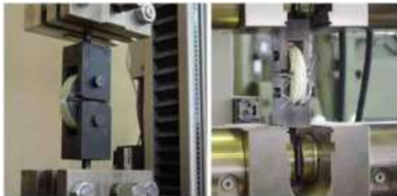
Figure 4: Universal testing machine: Zwick/Roell Z400 with max stress of 400MPa
