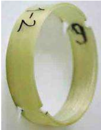
Figure 3: Illustration of the split-disk test specimen for tensile testing
