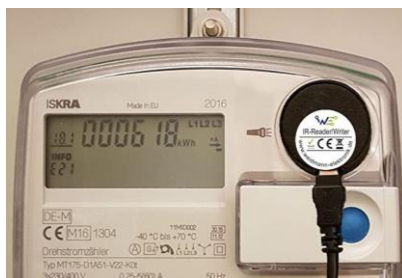
Figure 3. a) an SEM with connected optical IR sensor, and b) an optical sensor with IR-diodes (Rx and Tx).
