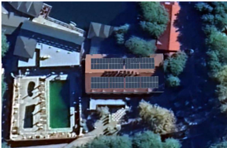
Figure 2. Visual presentation of the designed photovoltaic system
