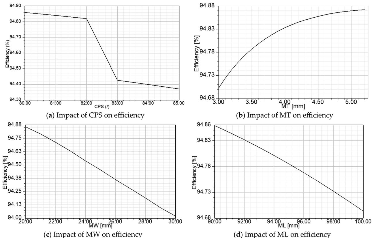
**Figure 10.** Impact of varied parameters on efficiency for M2-4 motor.
