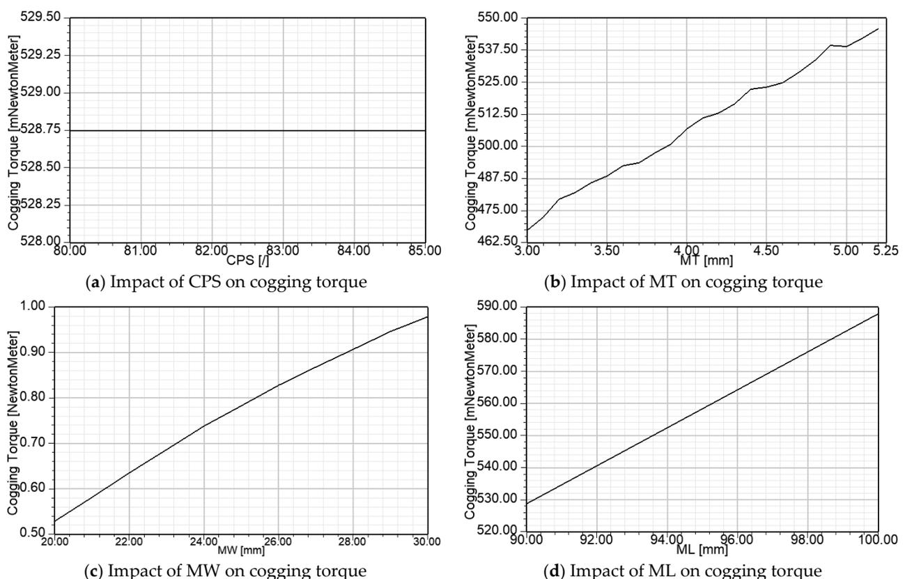
Figure 11. Impact of varied parameters on cogging torque for the M2-4 motor.
