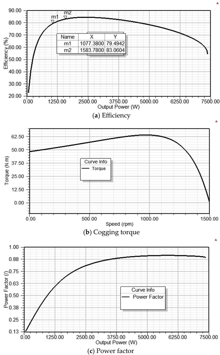
Figure 7. Steady-state characteristics of AM.
