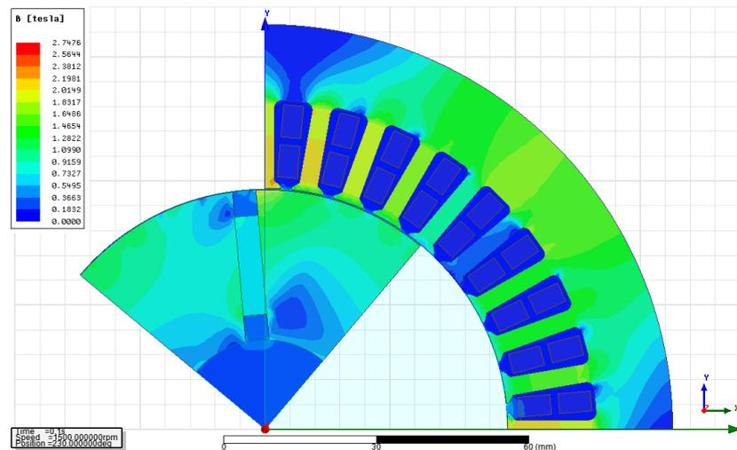
**Figure 5.** Flux density distribution at M2-4.
