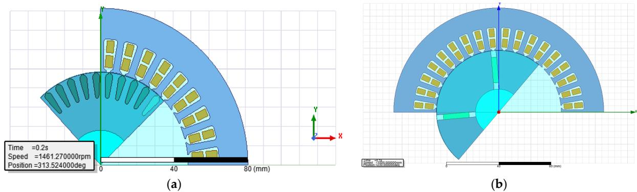
**Figure 1.** Motor's cross-section (a) asynchronous motor (b) spoke-type synchronous motor.
