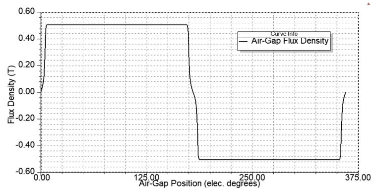
**Figure 4.** Air gap flux density distribution at M2-4.
