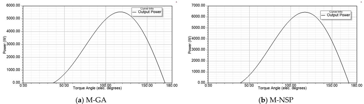
**Figure 9.** Output power of M-GA and M-SNP.
