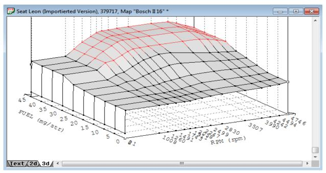
Fig. 14. Modified control surface for the pressure in the intake manifold
