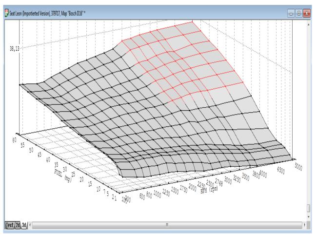
Fig. 12. Modified control surface for quantity of injected fuel
