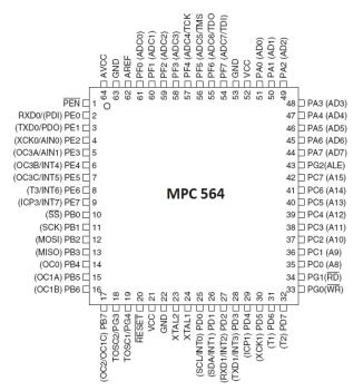
Fig. 1. Motorola MPC 564 microcontroller housing pin layout
