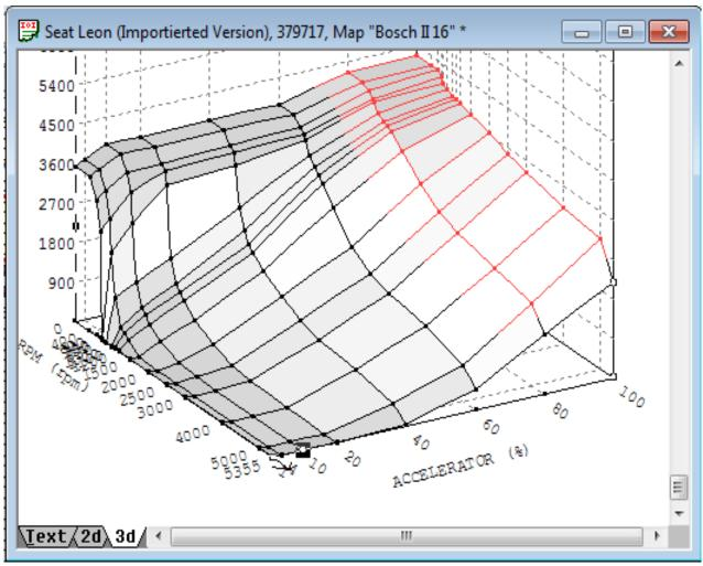
Fig. 4. Modified control surface for the accelerator pedal position
