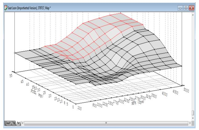
Fig. 10. Modified control surface for the moment of fuel injection
