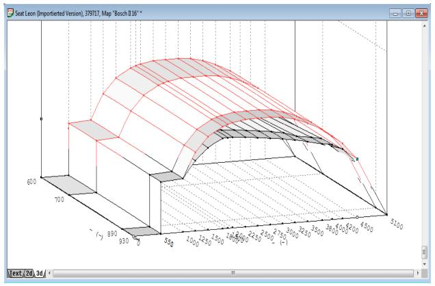
Fig. 6. Modified control surface to limit the torque
