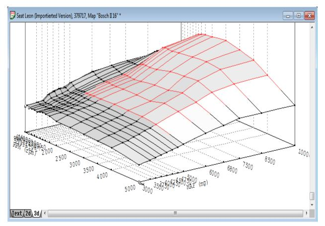
Fig. 2. Modified control surface for the control of the quantity of fuel dependent on the fresh air intake
