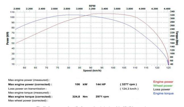
Fig. 2b. Power output for a "Performance" optimization of the SEAT Leon engine
