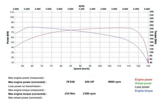
Fig. 2a. Power output of the non-optimized SEAT Leon engine
