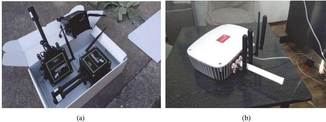
Fig. 4. (a) The 3 WaspmotePlug&Sense Sensor Nodes; (b) One of the Meshlium Multiprotocol Routers
