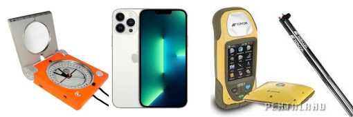
Figure 3. Used hardware: a) Klar compass b) iPhone-13 pro c) GPS Topcon GRS 1
