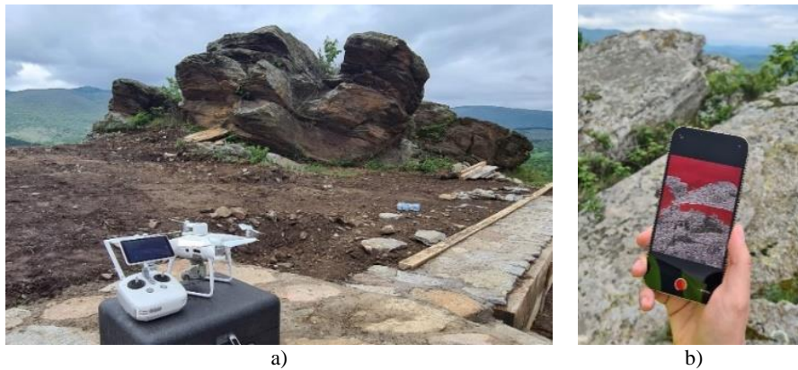
Fig. 2. Scanning: a) with drone b) with iPhone
