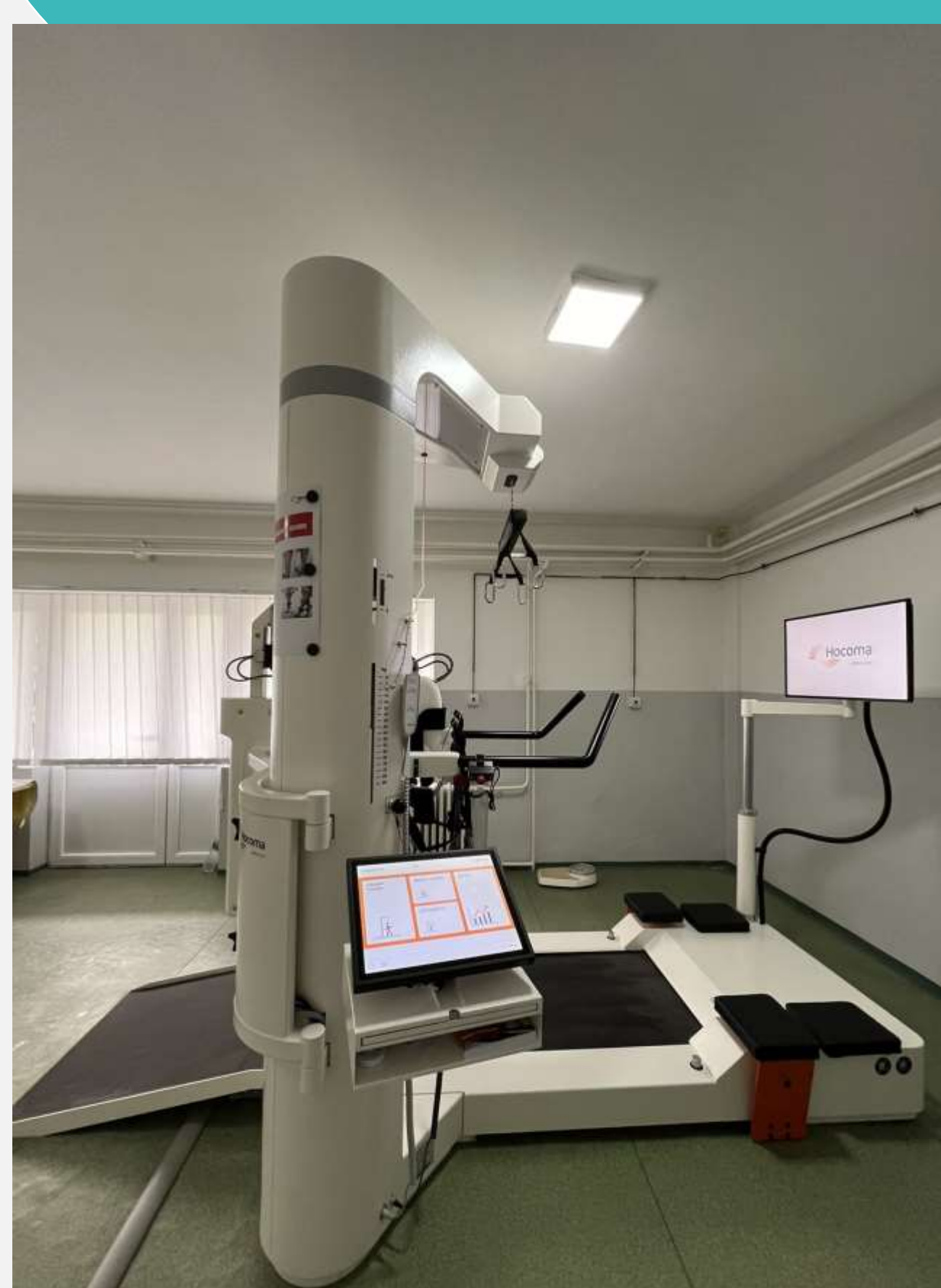
Figure 5. LokomatPro – a robot-assisted exoskeleton for the rehabilitation of lower limbs
