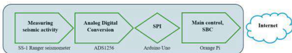
Figure 2. DAQ system general block diagram.
