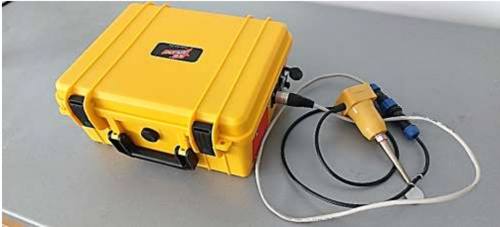
Figure 3. Prototype of DIY seismic DAQ station
