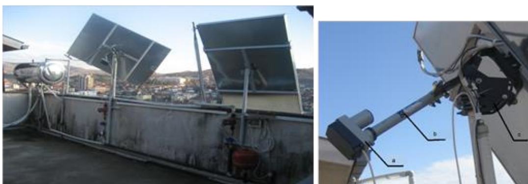
Figure 1. Experimental set-up and a segment of the tracking system: electric drive (a), gear spindle (b), auxiliary mechanism (c)
