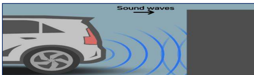
Figure 2: "Enhancing safety during reverse parking: Ultrasonic sensors.
