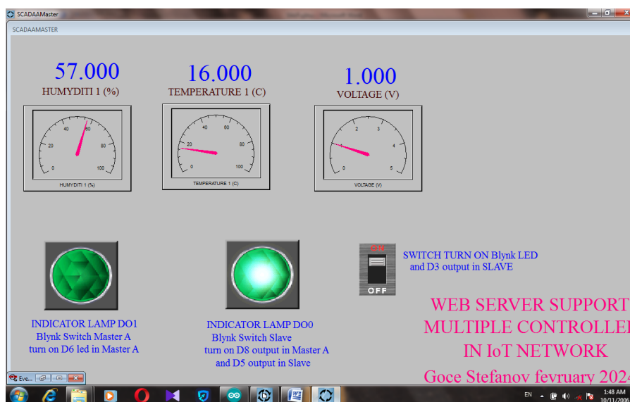
Figure 9. SCADA data system screen with defines variables
