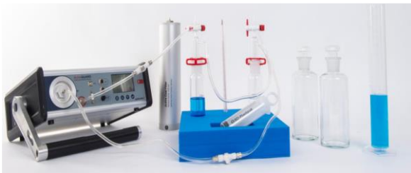
Fig. 3. a) Scheme and b) illustration of radon in water concentration experimental setup. The diagram shows the position where temperature and pressure are monitored. Attention should be paid to tubes length and internal diameter when computing the inner volume of the whole apparatus. (Saphymo GmbH, 2017)
