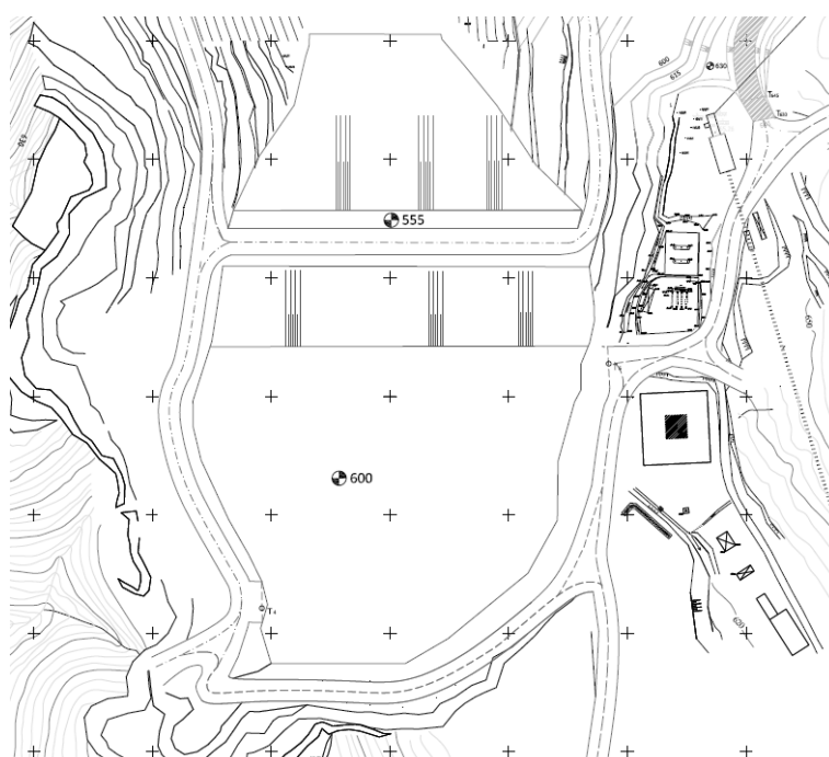
Fig 2. Formation of internal dump -Phase 2
