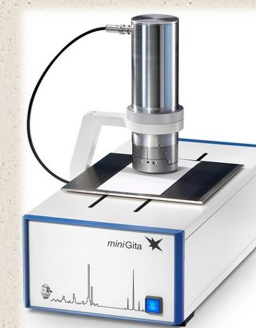
Radiochemical purity: Raytest miniGITA TLC scanner.
