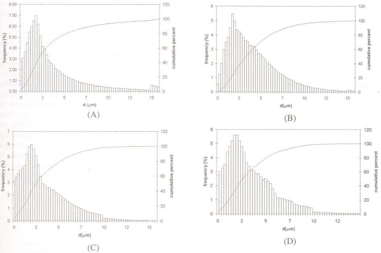
Fig. 1. Particle size-frequency distribution curves and cumulative distribution plots for series A, B, C and D
