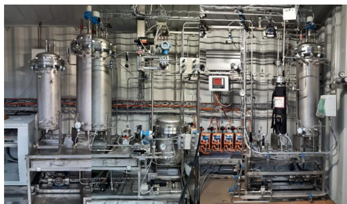
Figure 2: Layout of the electrochemical unit for OCEAN project
