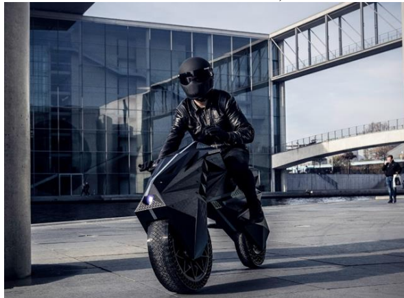
Figure 3. BigRep's NERA e-motorcycle features 3D-printed custom seats and airless tires (Natashah, H. 2018, November 26).
