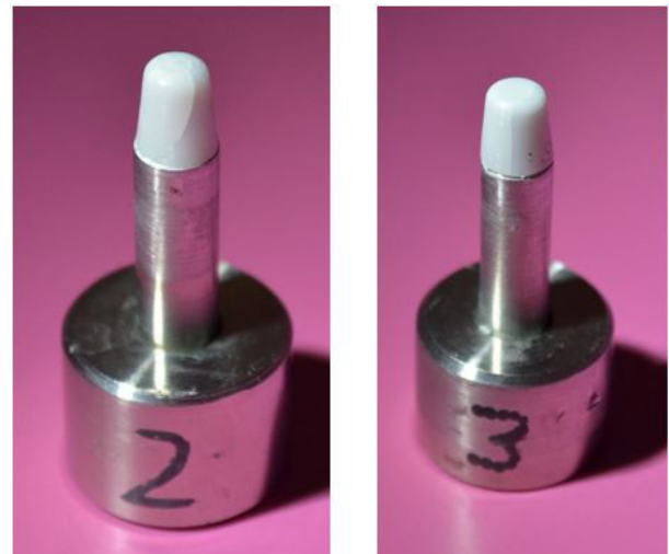
Figure 4. Fracture on zirconia copings after applying the load
