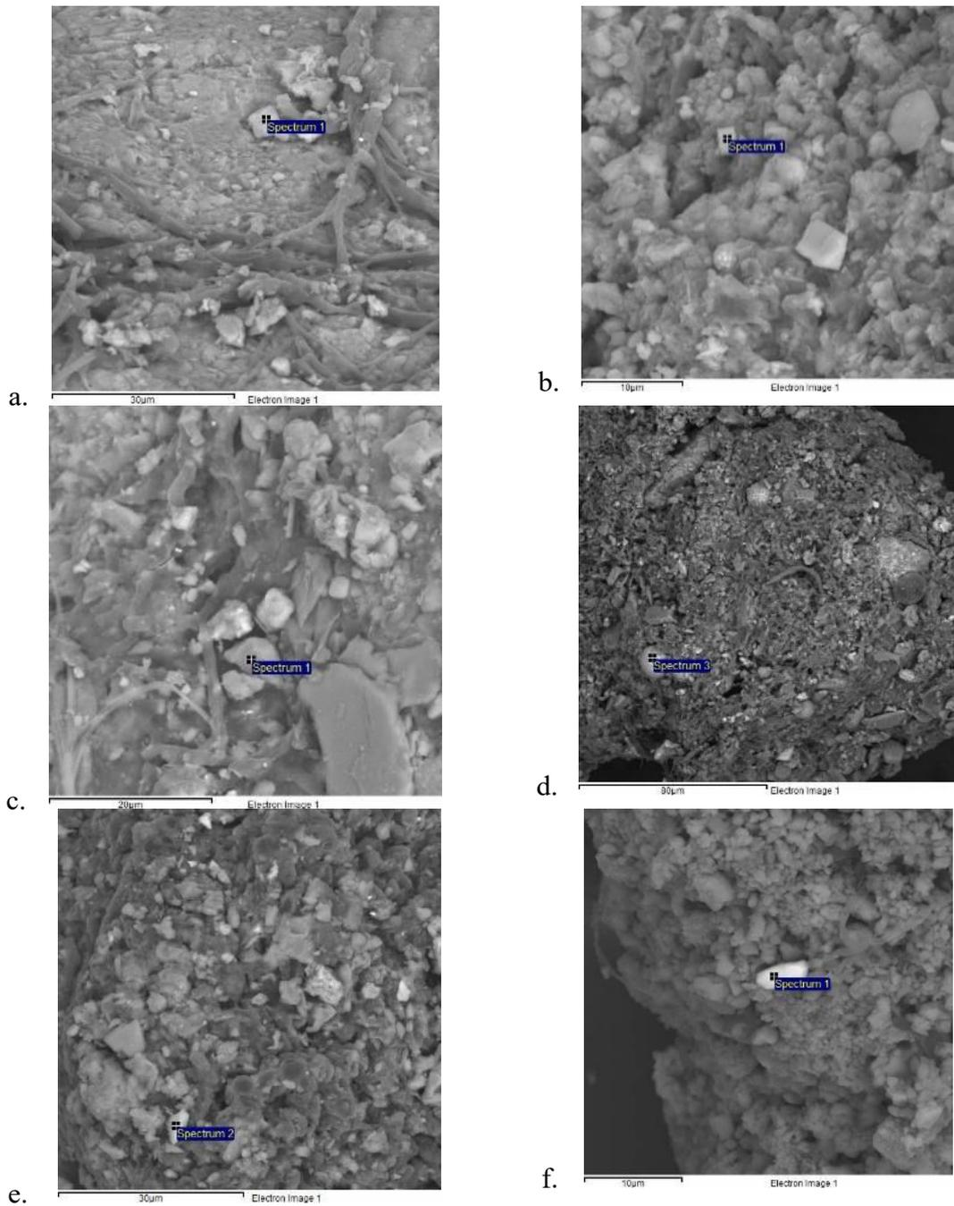
Figure 6. The SEM microscopic image of: a) feldspar; b) calcite; c) quartz; d) Fe, Mg silicate; e) Fe-oxides; f) zircon
