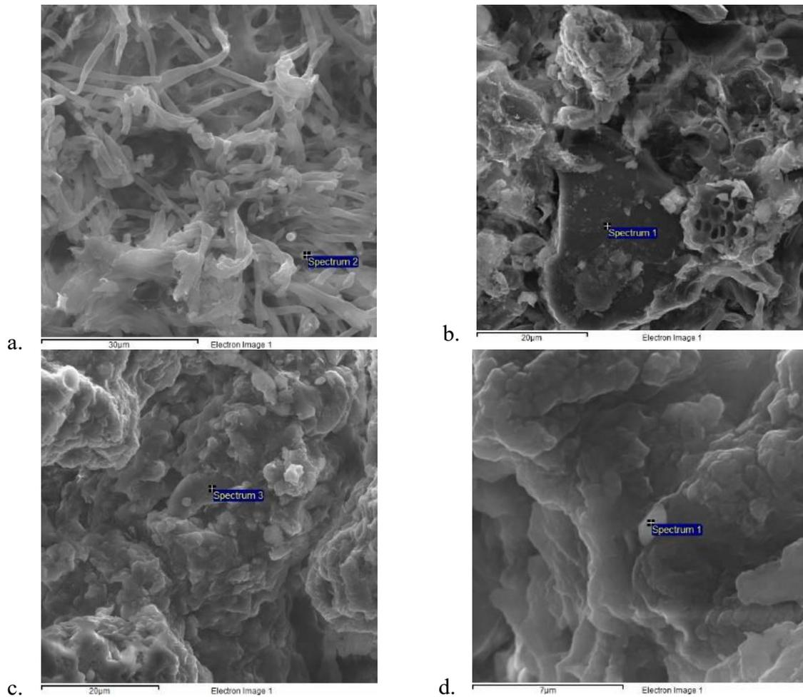
Figure 4. The SEM microscopic images of a) calcite; b) quartz; c) K, Al silicate; d) Ca, Al silicate
