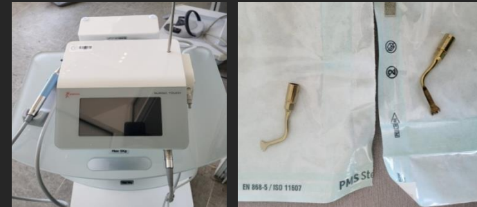
piezosurgery device and bone cutting attachments
