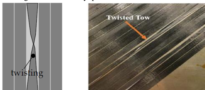
Figure 4: Schematic and actual representation of a twisted tow within a ply
