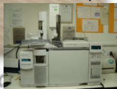
Agilent 5975 Mass Spectrometer coupled to an Agilent 6890N Gas Chromatograph
