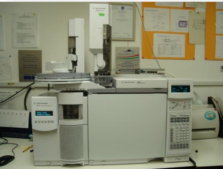
Agilent 5975 Mass Spectrometer coupled to an Agilent 6890N Gas Chromatograph
