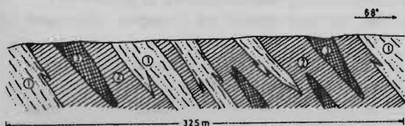
Fig 7. Cross-section through the Dolga Poljana ore occurrence 1. strip shaped micaceous gneisses, 2. poorly ore mineralized amphibolites and amphibolitic schists ( Fe < 10\% ); 3. ore bodies with increased concentration of Fe-Ti minerals ( Fe > 10\% )
