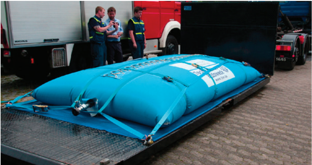
Fig. 2: A fresh water "bubble" installed by the Federal Agency for Technical Relief (THW) Bremerhaven (source: https://www.thw-bremerhaven.de/aktuelles/aktuelle-meldungen/artikel/trinkwasser-fuer-600-menschen/ ) © THW Bremerhaven
