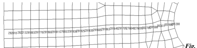
Fig. 6. Network of spring calculation. The network of the spring is divided into 21 parts and for each part is measured the stress on the underside of the spring.
