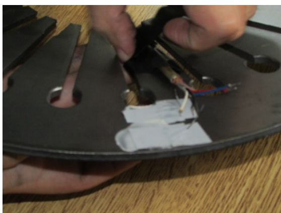
Fig.10a. Diaphragm spring with measuring tapes
