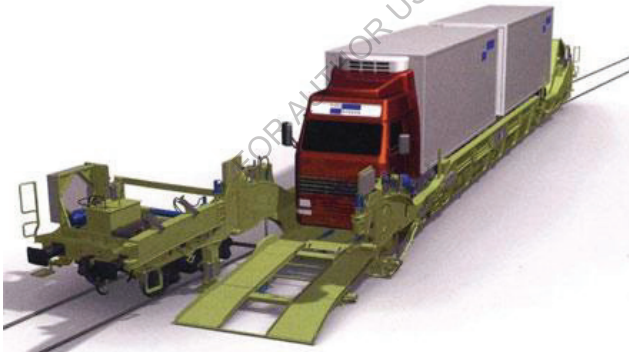
Figure 2: Unloading a truck with a trailer from a plate wagon 12
