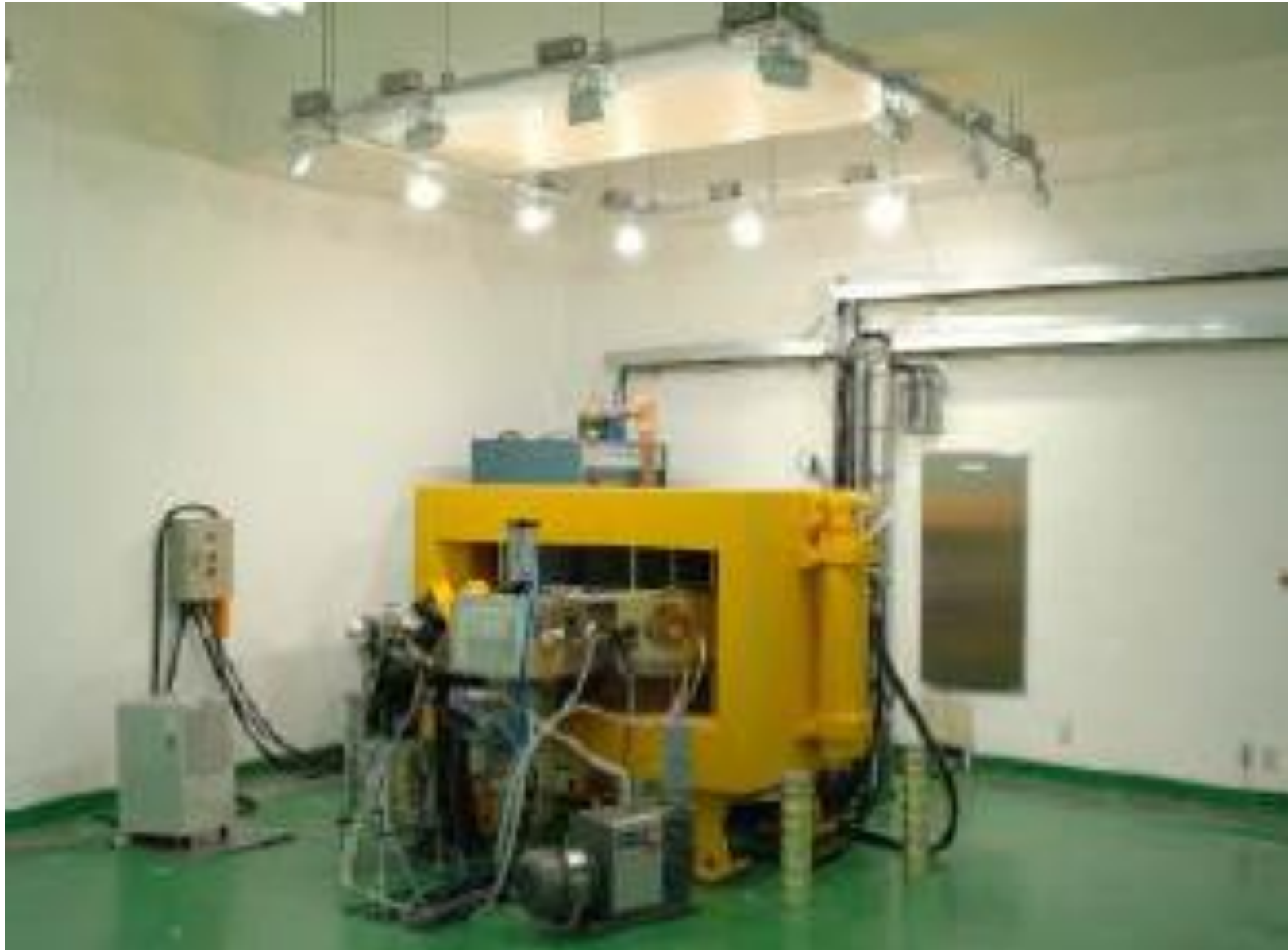
13 MeV cyclotron (indigenous product) in operation in Chosun University, Republic of Korea
