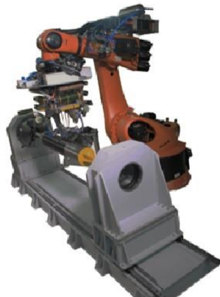
Fig. 6. In situ consolidation with LAFP head (Mikrosam D.O.O.).
