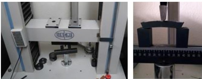
Fig. 7. UTM (universal test machine) and ILSS test (samples No.1 mounted on two supports)
