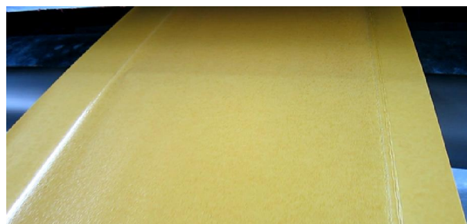
Fig.4. The oven - Resin film after oven
