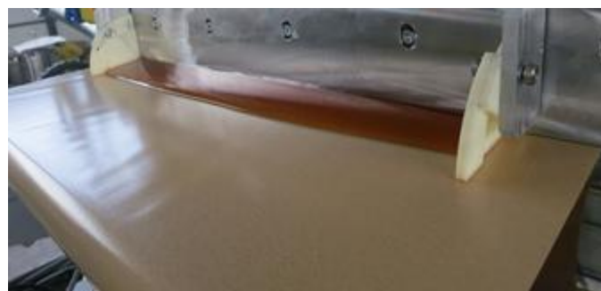
Fig.2. Knife – gap for thickness of resin film
