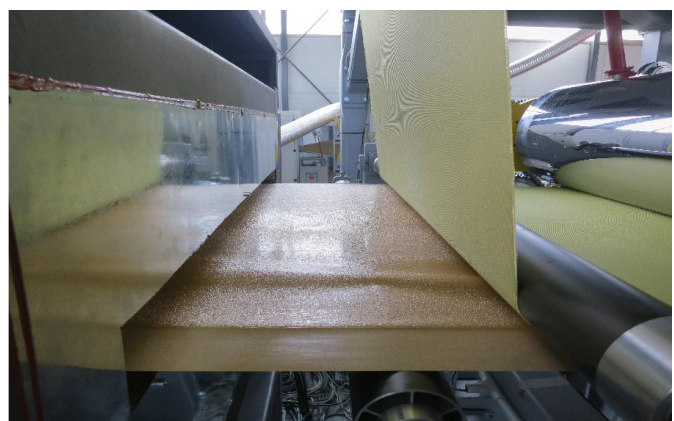
Fig.5. Resin film after oven and Kevlar fabric
