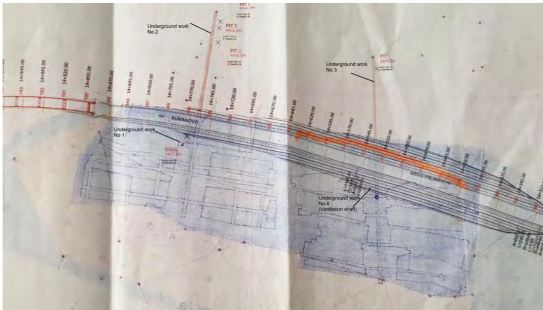
Figure 2. Plan of the actual condition of the underground mine for bentonite clay and location of the express road
