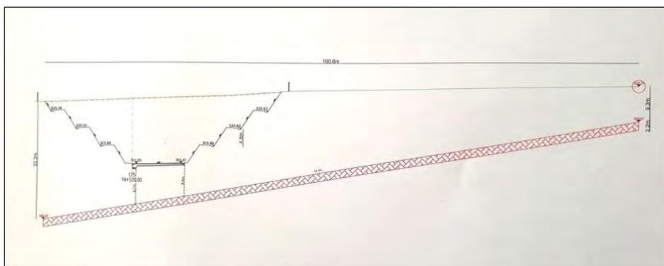
Figure 5. Estimated Location of hoisting decline No. 2 in relation to final road condition
