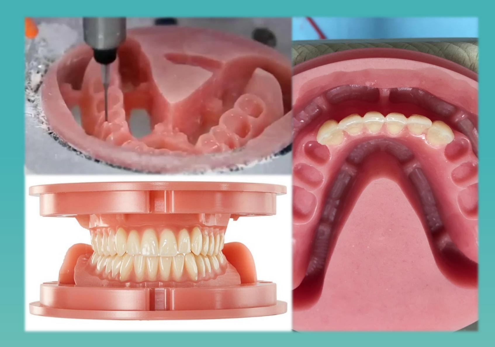
The material for digitally produced, are tooth coloured discs made from acrylic material, which are suitable for the individual design and production of whole tooth segment. The long-lasting dental restorations are individually customized to integrate with patients natural antagonist teeth
