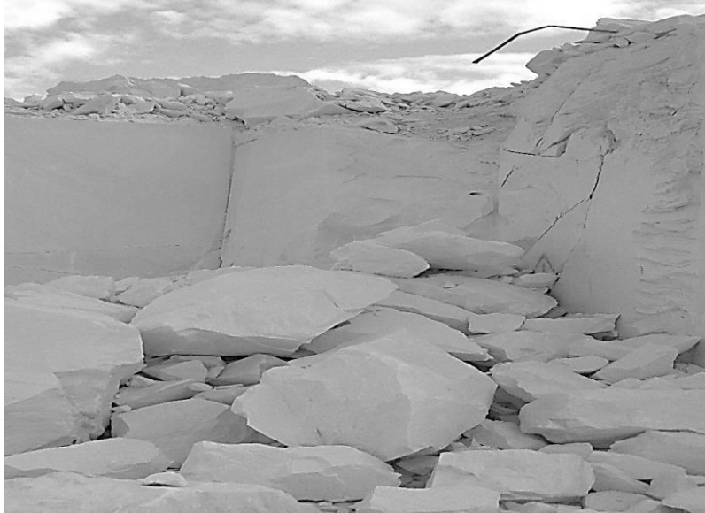
Figure 3. Blasting effects relative to granulometric composition
