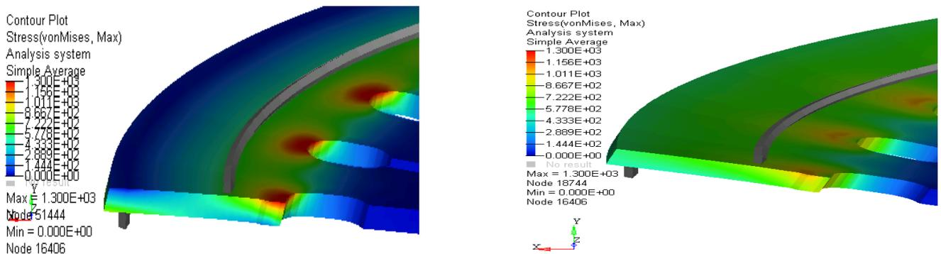
Fig.9 Complex stress at the flat and disengaged position Ø392/336
