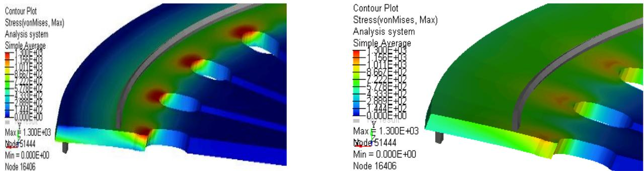
Fig.8 Complex stress at the flat and disengaged position Ø392/0
