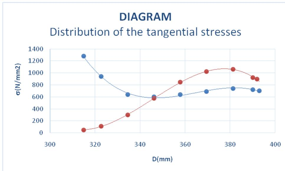
With one support \_\_\_\_\_, with two supports \_\_\_\_\_
