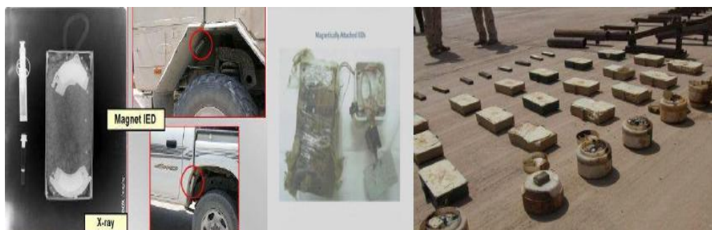
Picture 8 - Examples of magnetically attached improvised explosive devices and their setting
