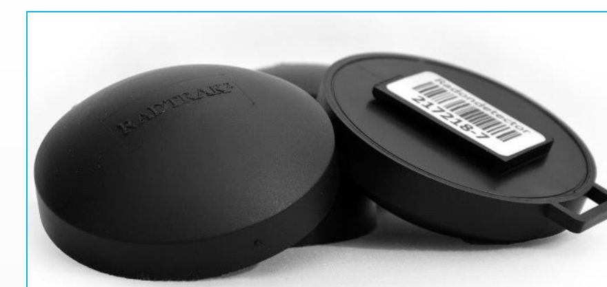
Figure 2: CR-39 nuclear track detectors used in the survey
