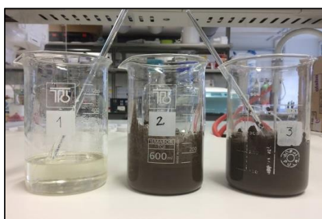
Figure 2. Illustration of the epoxy resin system, fly ash and mixture systems epoxy/fly ash
