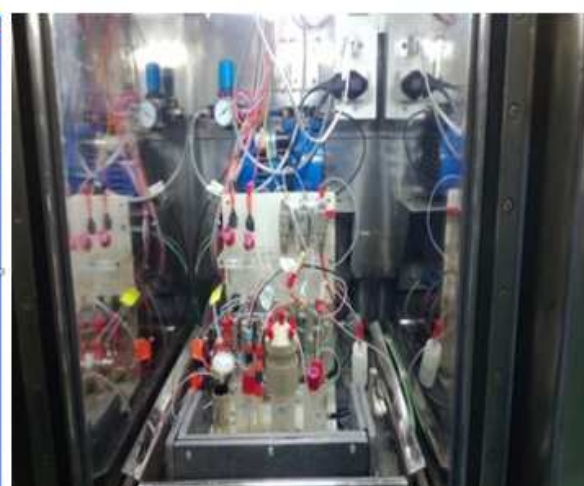
Figure 1: HMI Software for the \text{Na}^{18}\text{F} synthesis module Figure 2: \text{Na}^{18}\text{F} synthesis module inside the hot-cell
