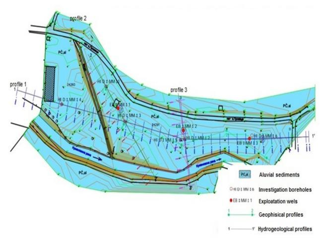
Fig. 3. Hydrogeological map with presented boreholes and wells at a locality "Mitev Most"
