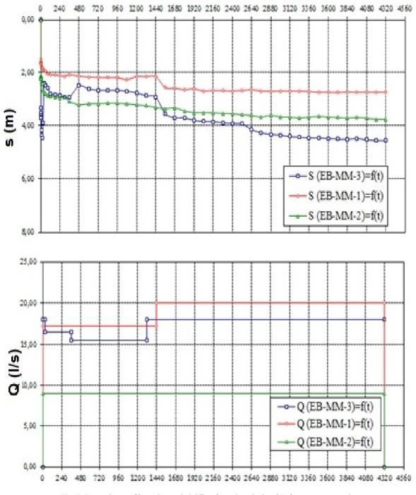
Fig. 7. Dependence of lowering and yielding from time S, Q = f(t) from group pumping
