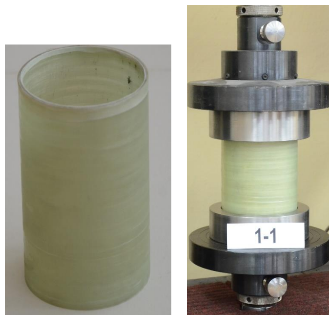
Figure 2. Illustration of the assembled tensile and compression test fixture and specimens
