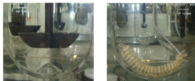
Figure 1. Photographic image of Peak™ vessel (left) and crescent-shaped spindle (right).
